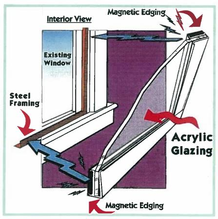
The magnetized gasket on your refrigerator door seals tight to keep the cold air inside. Magnetite® windows also seal
